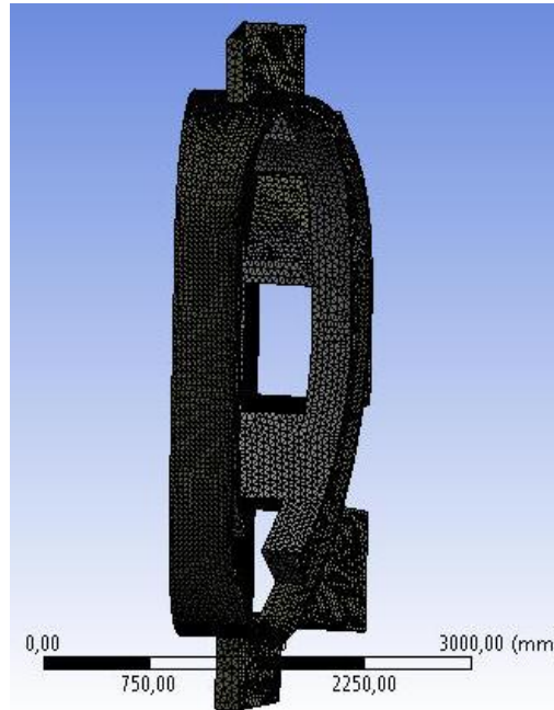
Figure 4.68: Mesh of DTT FW and VV single sector
